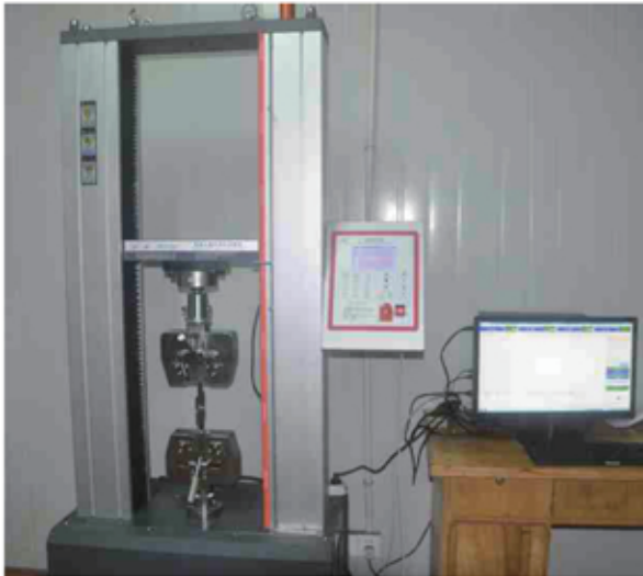
Computer Controlled Pull-off Tester (To Examine Welding Performance of Weld Zone )
