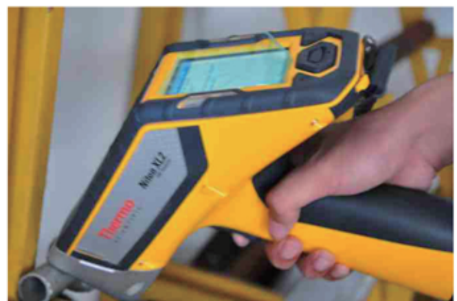
Portable PMI Tester PMI:Positive Material Identification
